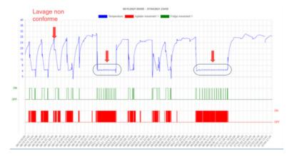
The monitoring of the evolution of the water temperature of the washing process made the detection of the nonconformity of the operation possible on a real-time basis.
