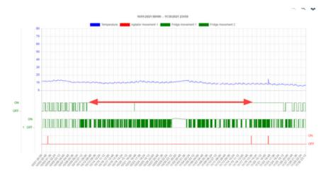
Diligent monitoring of the compressor activity led to the detection of a waste of energy: The compressor was on for a long period of time when it was supposed to be off.
